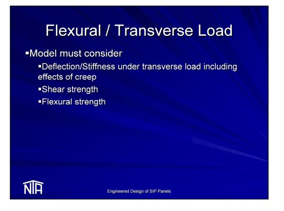
Based on basic engineering principles any model for SIP behavior under transverse loads must consider the following:
