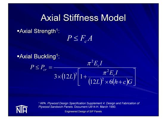
Based on the referenced documents, proposed equations for axial strength and stiffness are provided.
