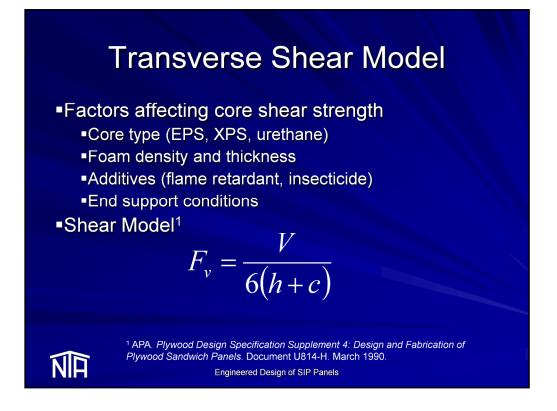
Moving on to transverse shear, known factors affecting the core shear strength include: core type, density, thickness, additives, and end support conditions. From basic engineering mechanics, the shear stress in a SIP can be expressed as shown in the equation provided. Using ASTM E72 ultimate load data from panels failing in shear (nearly all panels tested with simple supports) the ultimate shear stress *Fv* can be calculated.
