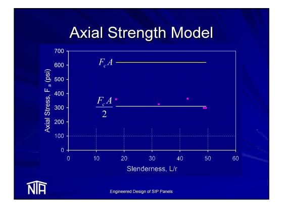
Returning to the axial load plot, the secant formula appears to accurately predict SIP panel strength under eccentric loading.
