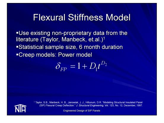
A literature review yielded a single comprehensive creep study on SIP panels. The study, conducted in the 90's, tested a large number of samples from 4 different panel manufacturers. The study considered EPS and urethane cores of various thicknesses (3.5 to 7-inches in thickness). The data cover a load duration from zero to 6 months for EPS and zero to 3 months for urethane.
