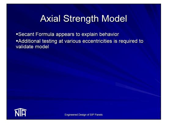
While the secant formula appears to model axial behavior, few tests have been run at eccentricities different than that required by ASTM E72. Testing at additional eccentricities may validate the use of the secant formula for other eccentricities commonly found in design, such as balloon framing where the eccentricity equals half the panel thickness.
