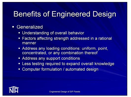
The benefits of this approach are many. Most importantly, this approach provides a understanding of overall panel behavior. It allows us to see the big picture. As part of this, factors affecting strength are addressed in a rational manner. And, because the models are based on engineering principles the models are "generalized", meaning that analysis can be performed to address any loading or support conditions regardless of what was tested.
