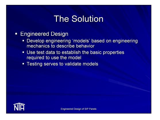
The solution to this problem is "engineered design". This approach requires the development of engineering formula's, or models, to describe the behavior of SIP panel in general terms. Once the models are established, test data are used to establish the basic properties required to use the models. Instead of the existing "design by testing" philosophy, the purpose of the testing is to validate the models.
