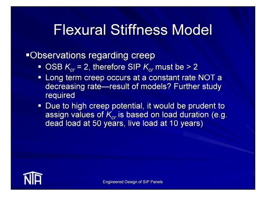
The Kcr for OSB is 2.0, because SIPs are comprised of OSB and foam plastic, the creep potential of a SIP would be expect to be greater than 2.0. Also, as previously mentioned, the long-term creep rate appears to be constant. This may be the result of the Power Model rather than actual creep behavior, but this would require more research at longer durations to assess.
