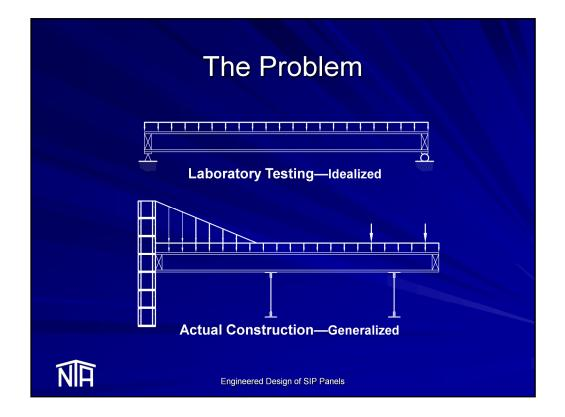
In the laboratory, specimens are tested under idealized conditions. For example, transverse load tests are typically conducted on full-size panels with simple supports and uniform loads (shown at top).
