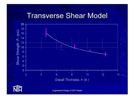
Plotting the shear stress verses the panel thickness, as shown in the plot, reveals that shear strength decreases as panel depth increases. This strength reduction is not accounted for by engineering mechanics but may be accounted for by a depth correction factor.
