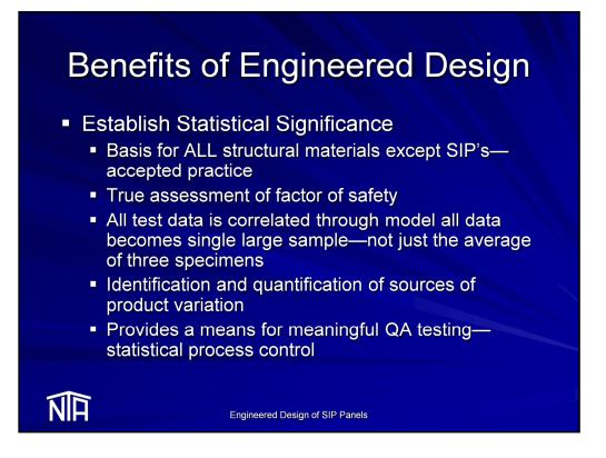
An additional benefit of engineered design that is less obvious is that it becomes possible to establish statistical significance. While "hidden" in the design procedures for common engineering materials, there is a statistical basis for all structural design. Structural loads are based on observed probabilities of occurrence and then adjusted to a required interval. While a material's ability to resist imposed loads is based on variability in strength and required strength confidence levels.
