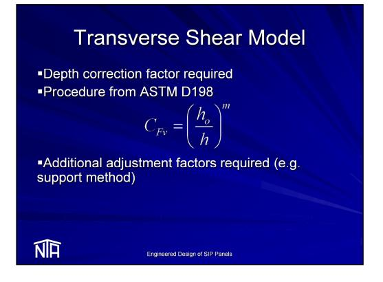
A basis for the formulation of such factors is provided in ASTM D198. The proposed equation expresses a shear depth correction factor,  $C_{Fv}$ , in terms of a reference depth,  $h_o$ , and the design depth, h. The curvature of the relationship is established by an exponent, m. Using simple curve fitting techniques m may be established for a given foam.
