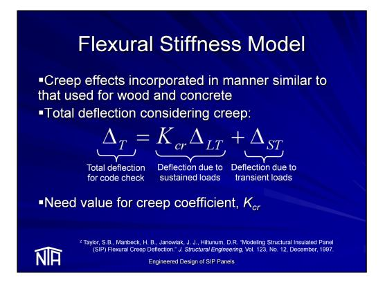
The stiffness model discussed so far considers only short term test loading, but in actual structures loads are applied for much longer periods. Accordingly, the long-term deflection under sustained loads must be addressed in a rational manner. As previously mentioned, all non-metallic materials creep under sustained load, the common design expression used to account for such behavior is provided.
