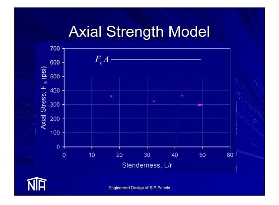
However, comparing the proposed models to actual data (as done in the plot) shows that the models do NOT reflect tested behavior—the tested strength is about ½ the strength predicted by the model.
