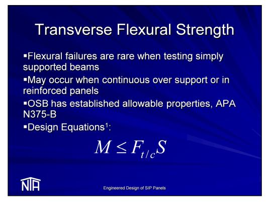
Looking at flexural strength. In general, tests on simply supported SIP panels exhibit shear failure at ultimate load NOT flexural failure of the facings. However, flexural failure may occur in panel continuous over a support or in panels with structural splines.
